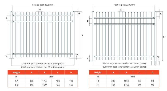
The Mercury Tubular Aluminium Security Panels And Gates - refer to spec sheet for more details.
