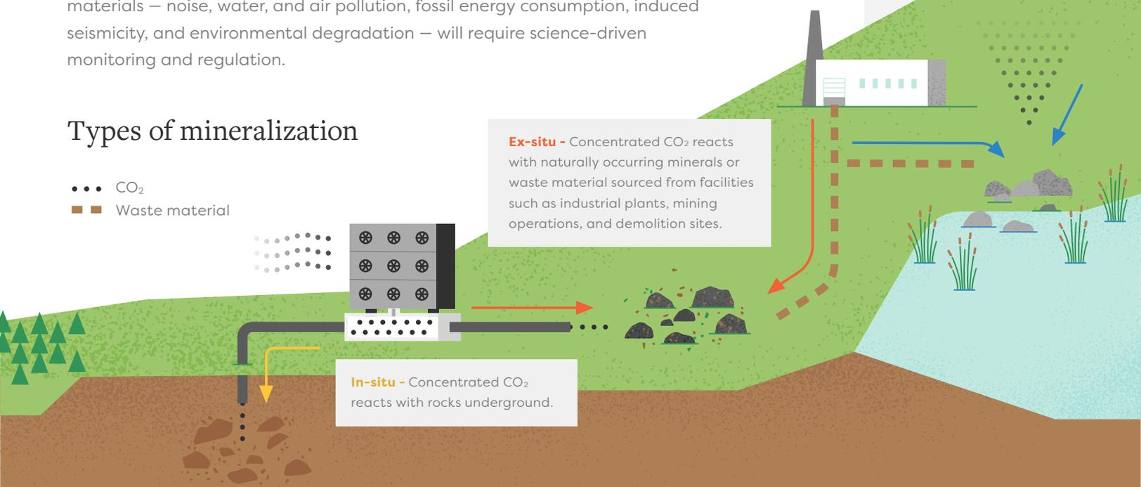
**Ex-situ** - Concentrated CO<sub>2</sub> reacts with naturally occurring minerals or waste material sourced from facilities such as industrial plants, mining operations, and demolition sites.
