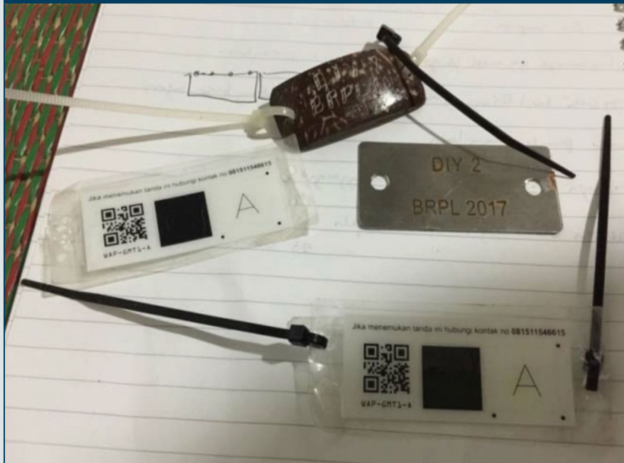
Tags tested during fishing gear marking experiment. Metal, bamboo and Septillion tags are shown here with cable tie attachments.
