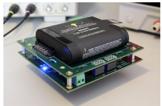
EDG's Cellular Controller and Smart Battery Charger
