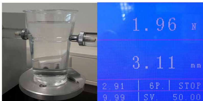
Figure 39: Cup Compression Tests instrumentation
