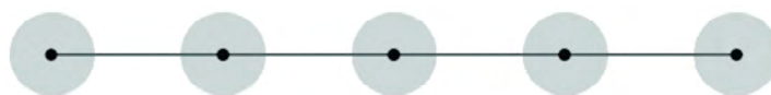
Figure 3. Schematic of a point-transect depicting a cluster of five, 1/5th acre plots spaced four chains (264 ft) apart upon which habitat metrics will be sampled.
