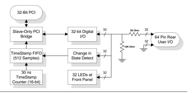
The Technobox 32-Channel Digital I/O board provides 32-bits of bi-directional CMOS-level (TTL compatible) I/O available at the JN4 connector on a PCI Mezzanine Card.
