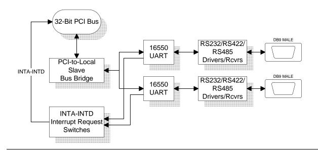
The 2-port Async Communications Adapter is a costeffective solution for providing additional RS232/RS422/ RS485 based serial ports for a host processor.
