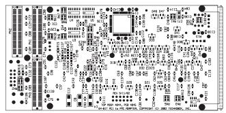
to buffer the PCI clock. The circuit allows positioning of the PCI clock edge +/-4 ns from the nominal position in 1 ns steps using a rotary switch on the board. This allows "tweaking" of the PCI clock to optimize setup and hold times on the PCI-X bus. The PLL operates up to 110 MHz.
