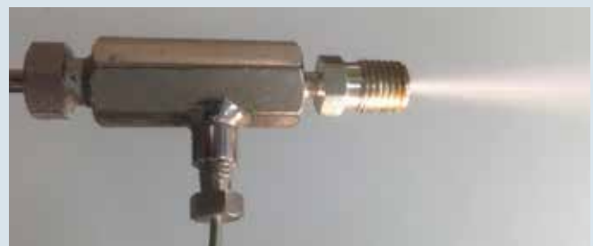
FIGURE 12. MARINE CLOUD BRIGHTENING SPRAY NOZZLE.
