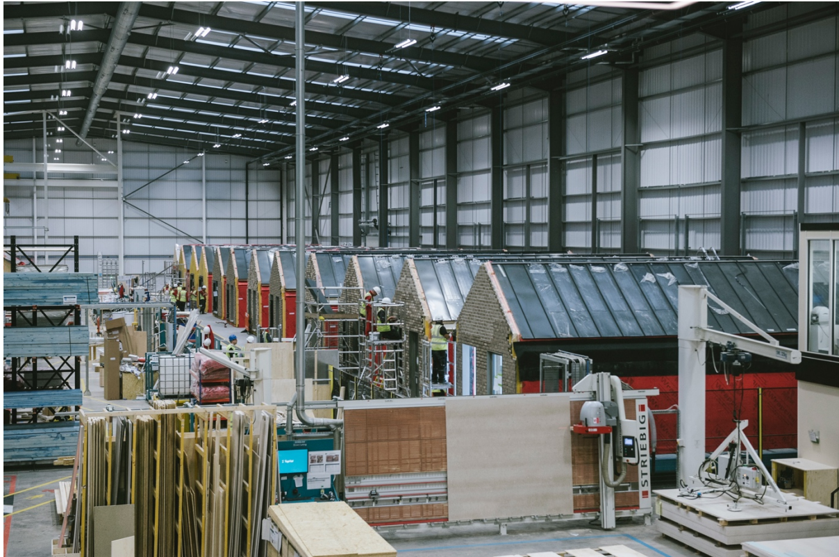
Figure 2: BoKlok homes on TopHat's factory finishing line, photo courtesy of TopHat Solutions
