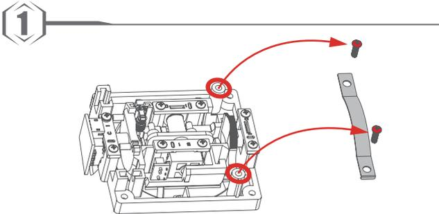
3. Take the transmitter apart, then remove the screws marked in blue and remove the bracket.
