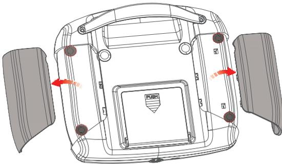
1. Use tweezers to remove the left and right hand grips. Then use a screwdriver to remove the 4 screws marked in red.
