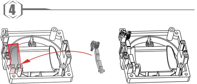
4. Place the spring hook assembly into position and hook the spring onto the hook located inside the transmitter.
