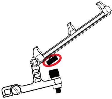
1. Loosen the locking screw by turning it anti-clockwise.
