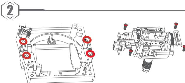
2. Loosen the screws shown in fig.4 and remove the plates.
