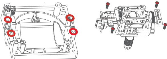
3. Loosen the assembly screws shown in fig.4 and remove the plate. Be careful to ensure no damage to cables.
