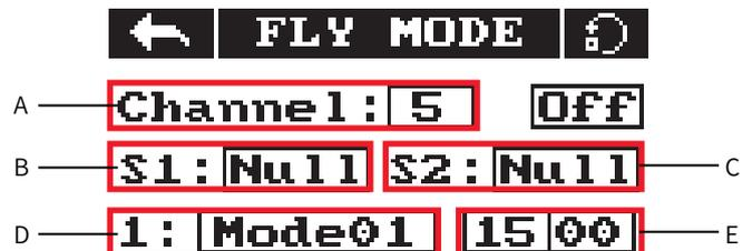
Different fly modes are assigned using combinations of switches. A 2-way switch will enable you to switch between modes 1 and 2, two 2-way switches will enable you to 4 fly modes, two 3-way switches will allow you to switch between all 9 fly modes. Use the table below to see which positions are assigned to each mode.
