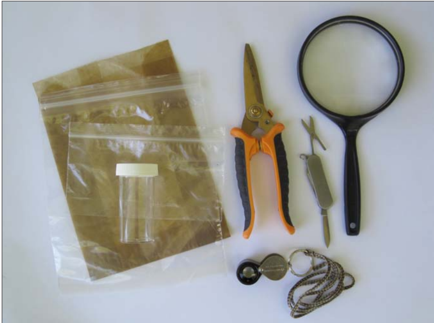
Figure 9. The right tools help with diagnostic work. Pictured here are cutters, sample containers, a magnifying glass and a 10× hand lens.
