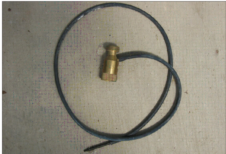
Figure 7. A simple hose-on-type proportioner is commonly used in a system for applying liquid fertilizer in a greenhouse.
