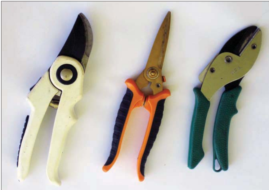
Figure 1. Hand shears come in two basic styles: bypass shears (left, center) and anvil-pruners (right). Bypass shears are preferred because they typically make cleaner cuts than anvil pruners do and don't crush twigs or branches.
