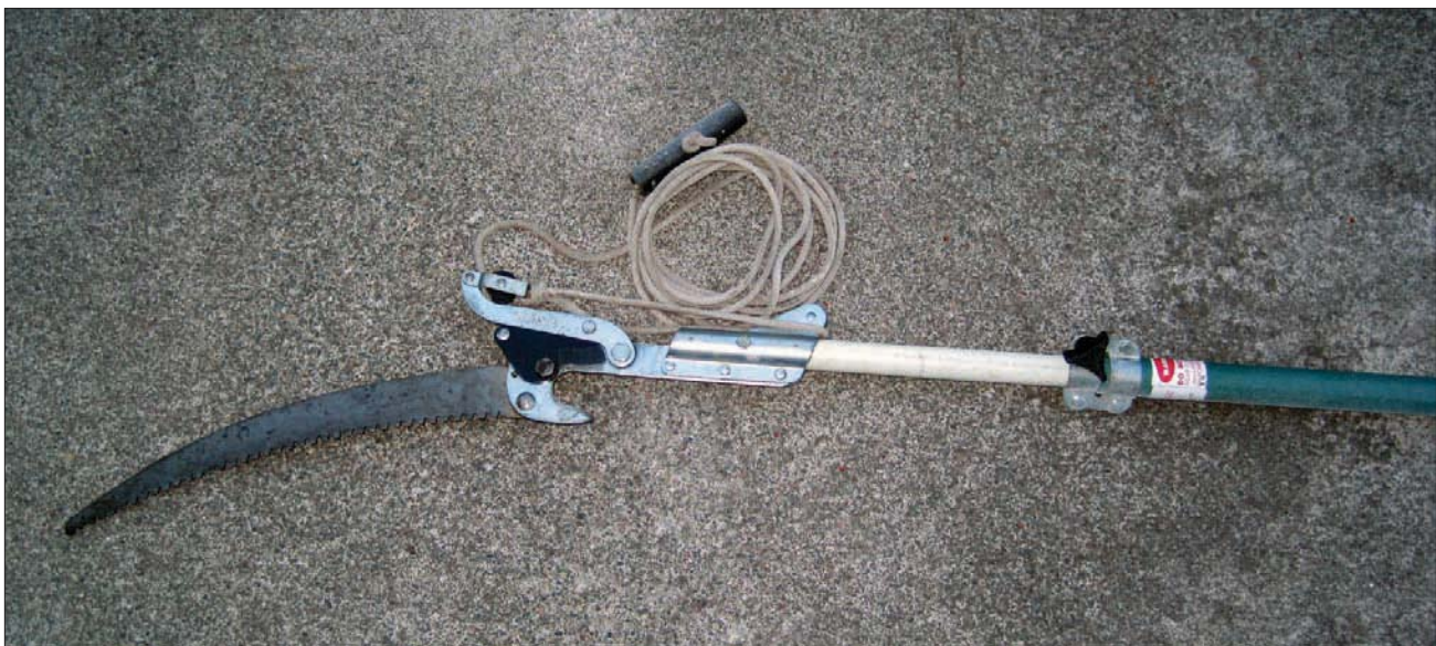
Figure 3. Pole pruners cut like loppers and may also have a saw blade for cutting larger limbs. Be sure to wear safety equipment when using a pole pruner, and be extra careful when working around power lines. Do not stand directly under the branch being cut with a pole pruner.
