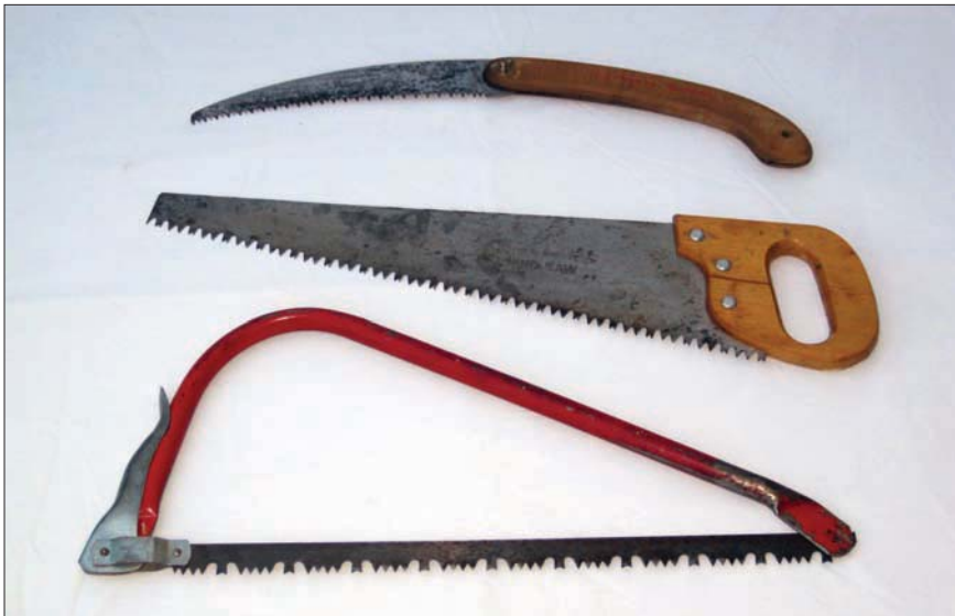
Figure 5. Pruning saws come in a variety of shapes and sizes and are useful for cutting branches or limbs between 2 and 4 inches in diameter.
