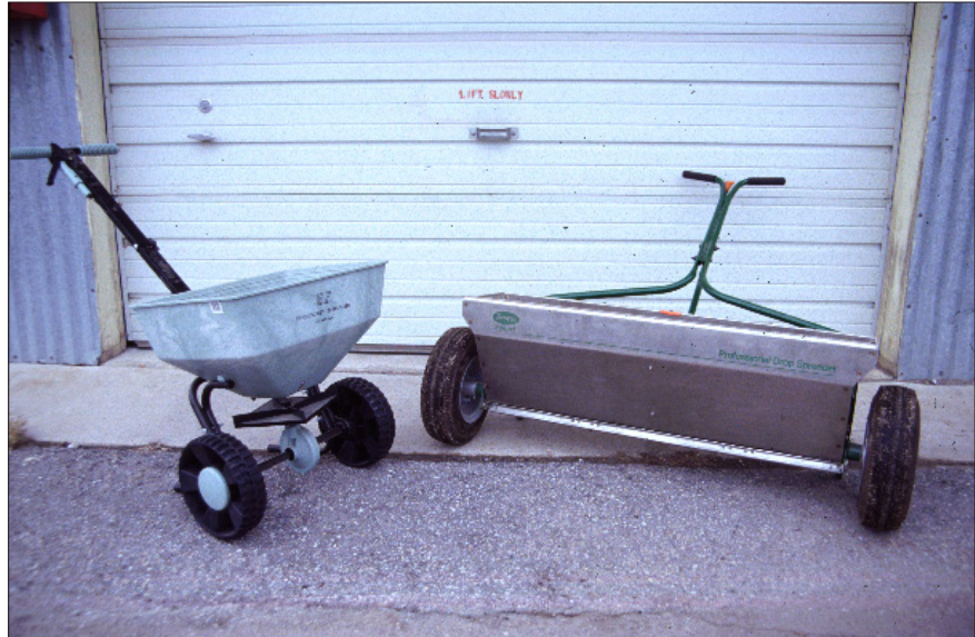
Figure 3. Two common types of broadcast applicators are the drop spreader (right) and the rotary spreader (left).
