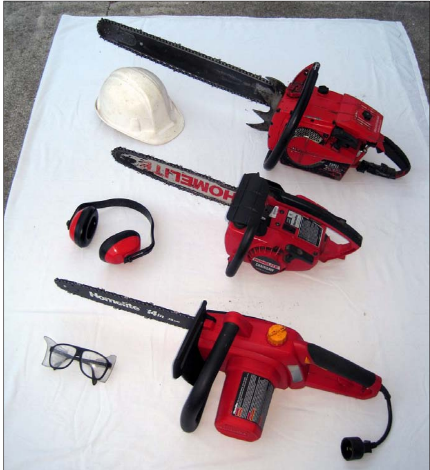
Figure 6. Chain saws come in a variety of sizes and styles. Use extreme caution and wear protective clothing as well as eye- and hearing-protection when using these power tools.
