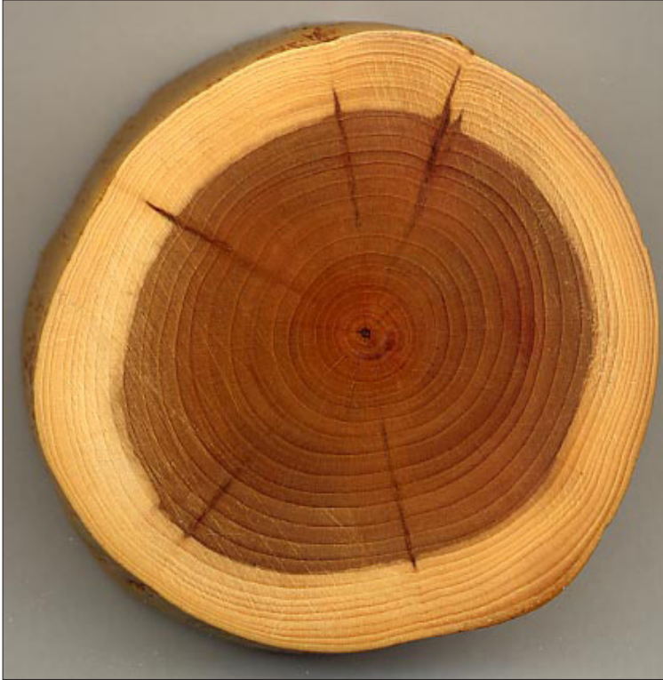
Figure 2. Section of a yew ( Taxus baccata ) branch, showing 27 annual rings, pale sapwood and dark heartwood, and pith (center dark spot). The dark radial lines are small knots—early branch stubs that were grown over by newer wood.
