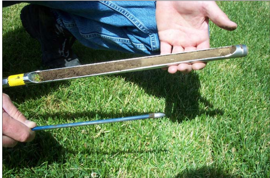
Figure 3. Both soil probe (top) and tile probe (bottom) indicate similar depths of water movement (about 6 inches indicated here).
