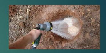
Once drained immediately refill the hole with water and measure the depth of the water with a ruler.
