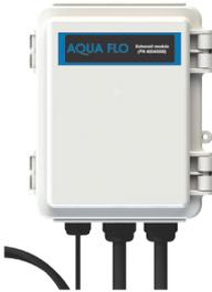
**SOLENOID CONNECTION MODULE:** Connects a NORMALLY CLOSED line voltage solenoid valve to the system. On a non-monitored system, the solenoid will only close on a lamp failure error. On a monitored system, the solenoid is closed when the UV level drops below 50%. Also note that in cases where emergency use of untreated water is required, the controller can be placed into a manual override mode allowing for the flow of water in an alarm condition. Order PN **40040006**.
