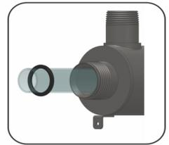
**Figure 4. Quartz Sleeve Installation**
