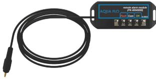
**REMOTE ALARM CONNECTION MODULE:** Allows for a connection to a remote device such as a buzzer, light, alarm system, PLC, etc., via a pair of contacts. In normal operation the OK and COM contacts will be connected, and in a fault condition (Low UV, Lamp fail, Power Fail), the Fault and COM contacts will be connected. Maximum Contact Rating is 1A-120V AC/DC (use 16-22 AWG). Order PN **40040008**.
