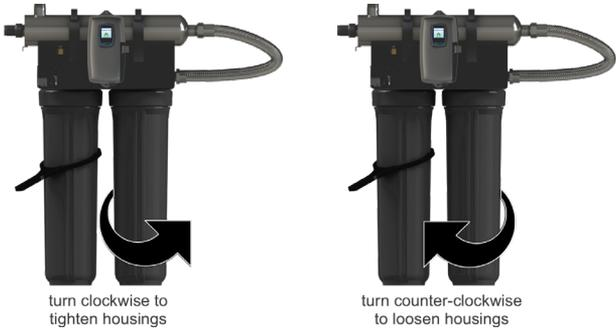
**Figure 5. Cartridge Removal**
