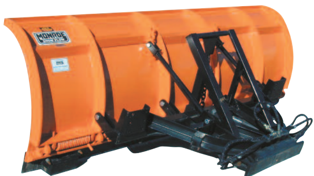
C-Style (6) Non-Adjustable 3/4" Square Torsion Spring Assemblies for a Bolt-On Trip Edge Assembly
