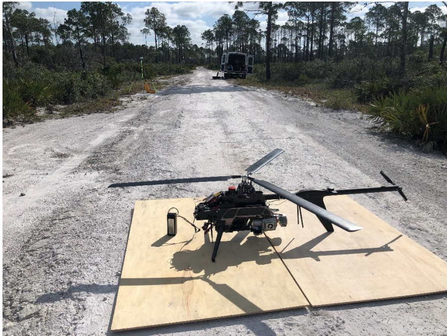
Figure 5: Riegl VUX-1LR lidar sensor and Sony A6000 camera integrated on a Pulse Aerospace Vapor 55 UAS platform. The picture here shows the platform without its cover.
