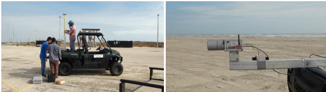
Figure 8. Example of the mobile lidar scanning system being mounted on an ATV near Packery Channel Jetty, Corpus Christi, TX. A similar setup was used at LSGI during the Summer 2019 field campaign by mounting the sensor on one of the ANERR’s ATVs.
