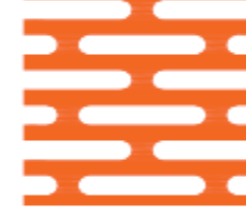
S1931SR 19.05mm x 3.18 mm Slots 41% Open Area
