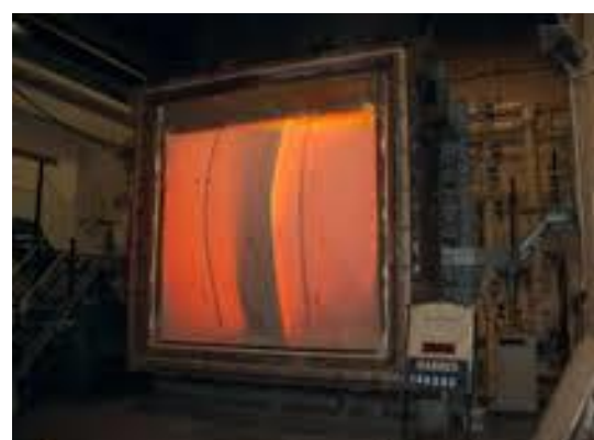
Figure 21 — Typical fire curtains being tested
