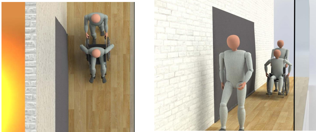
Figure 14 — Schematic showing needs of escapees passing a fire curtain
