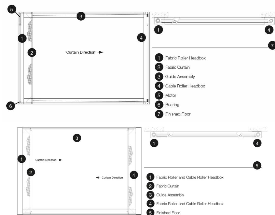
Figure 7 — Components of a horizontal fire curtain
