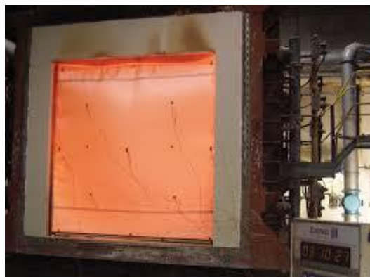
Figure 20 — Fire curtain being fire tested for integrity (E)
