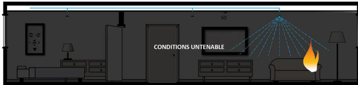
Stage 5: Although it cannot be guaranteed, sprinklers may extinguish fire - conditions remain untenable for any occupants who have not escaped at stage 2.
