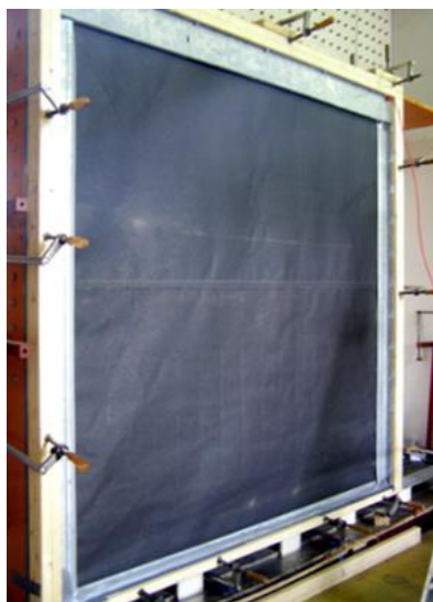
Figure 22 — Typical fire curtain being tested for smoke leakage
