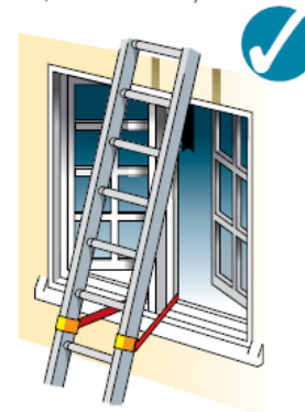
Figure 18a Ladder tied at top stiles (correct for working on, not for access)
