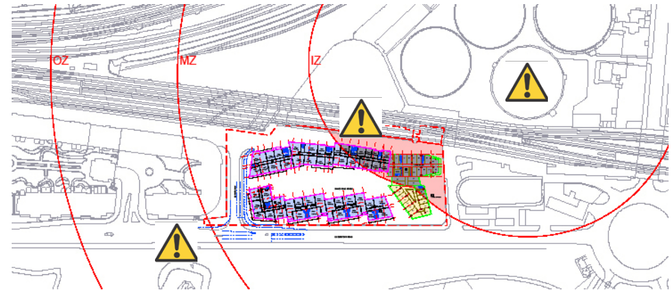
Site Plan with significant hazards indicated
