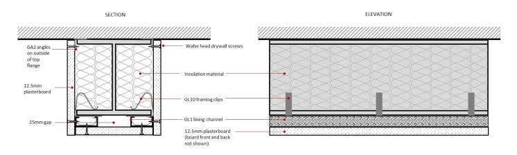
In each case the mineral wool tested was non-combustible (EN13501-1; A1) and had a minimum density of 40kg/m<sup>3</sup> and in each scenario the time for the test piece to reach the critical temperature (500°C for the columns and 576°C for the beam) was greater than for the respective control sample.
