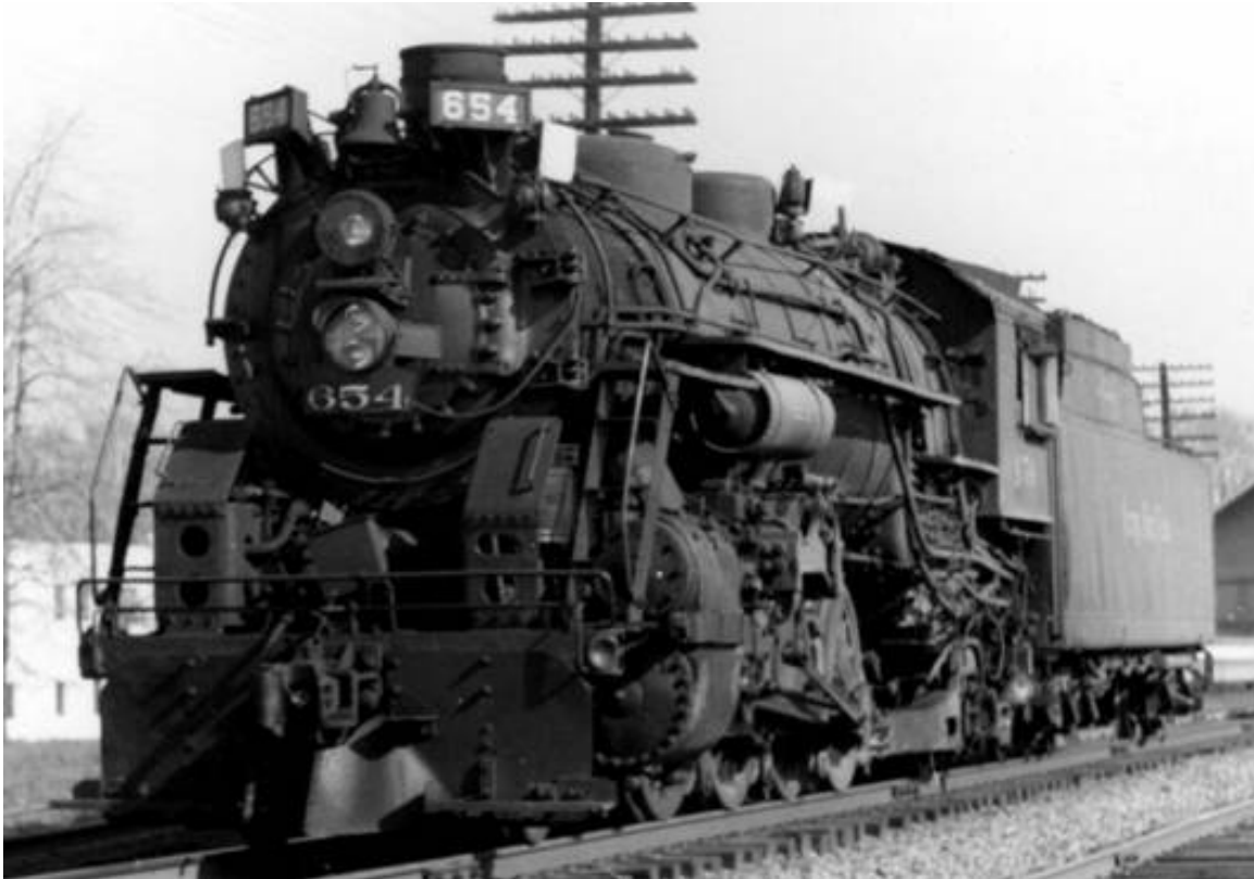
NKP 654, Painesville, OH, 10/1956. The engine has lost its booster and Worthington feedwater heater, and has a sheet steel pilot, multiple-bearing crossheads, and a Mars light. Without the Worthington and booster piping, you can clearly see most of the lower boiler.
