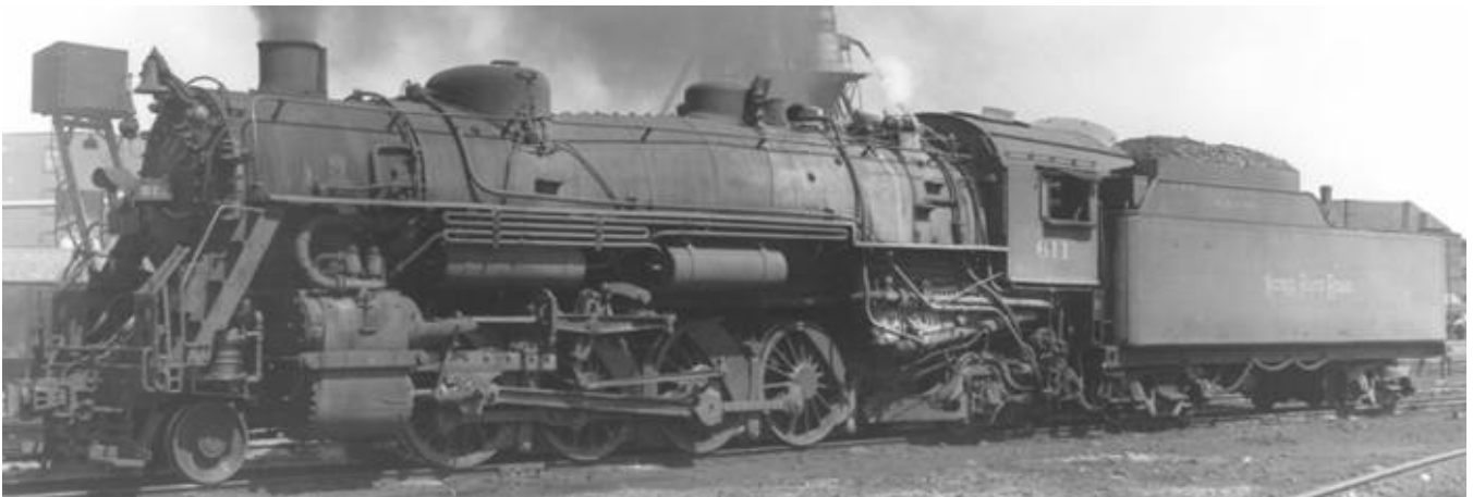
NKP 611, Peoria, July, 1941. The engine has had the multi-bearing crossheads added recently, but otherwise looks the same as it did throughout the 1930s. Surprisingly, while the NKP's records indicate that the 611 was fitted with a feedwater heater in April, 1922, the engine seems to have lost it during the Depression, while the rest of the class retained theirs into the 1950s.
