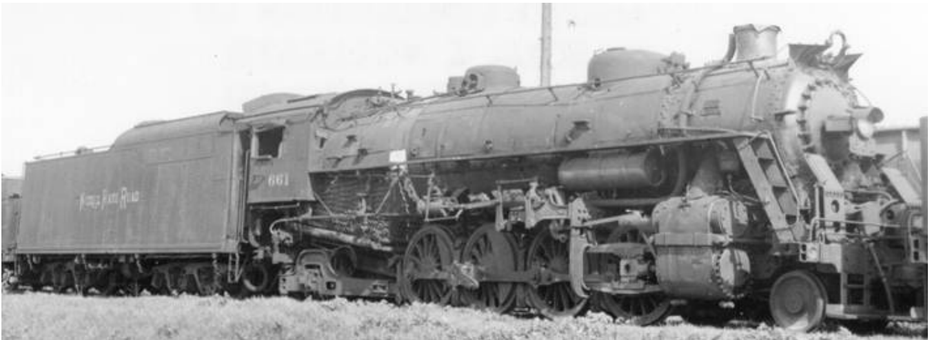
A stripped NKP 661, in the dead line at Bellevue, illustrating how the lack of major appliances makes the latter H-6e's look naked. The engine has been equipped with a footboard pilot.
