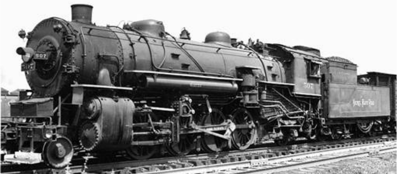
NKP 507 in the late 1940s. Notice the new footboard pilot and cab, as well as the cut back switching tender (added to engines serving as local switchers on the Chicago to Buffalo mainline).
