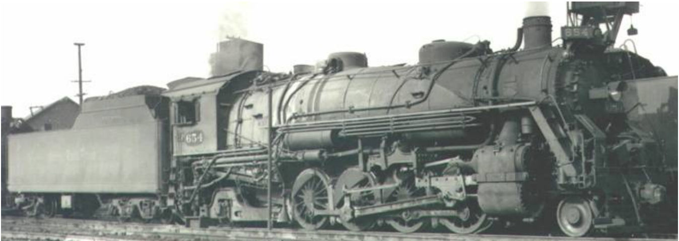
NKP 654, Peoria, 1949. The engine has received multiple-bearing crossheads, flying number boards, two extra sanding lines, and a stack extension.
