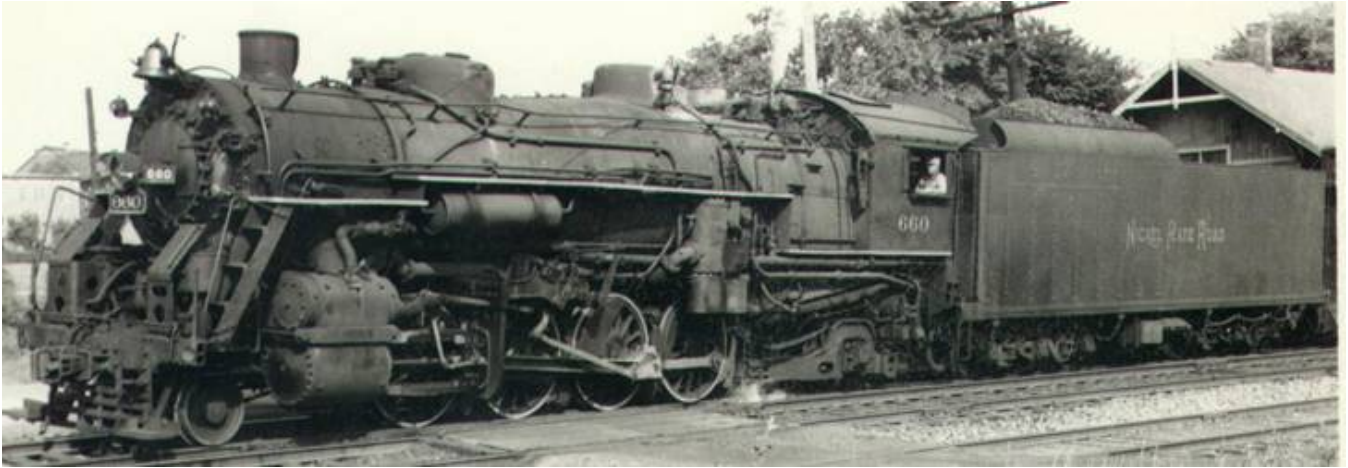
NKP 660, Valparaiso, 1949, showing what the fireman's side of the engines looked like after the air pumps were moved to the pilot deck.
