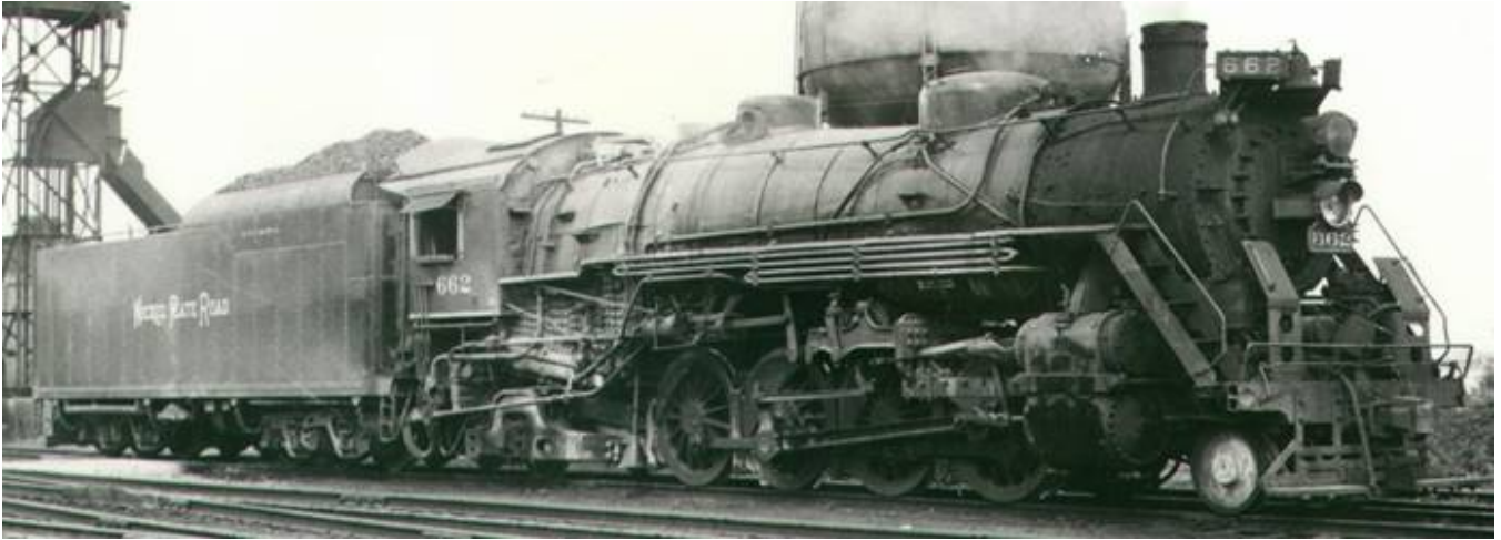
NKP 662, Madison, 1954. The engine has had the pilot truck whitewashed to check for cracks.
