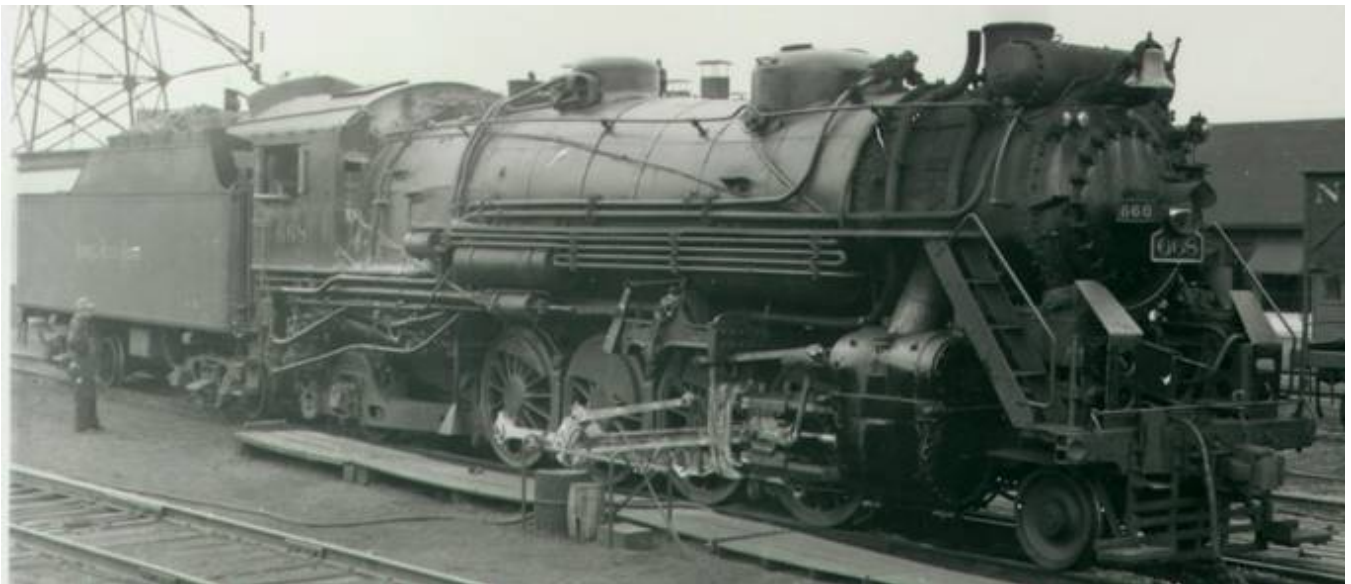
NKP 668, Conneaut, 1939. The engineer's side of the H-6f, once the air pumps were moved to the pilot deck.
