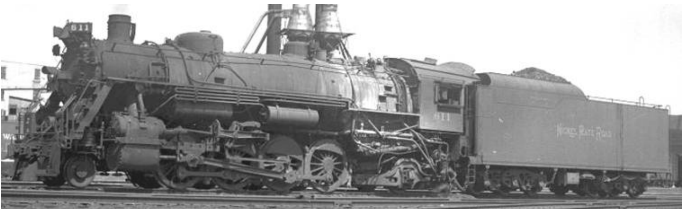
NKP 611, Peoria, March, 1948. Barely seven years later, 611 looks much different. The engine is now trailed by a 22RA tender (fairly common for the Peoria division), new piping arrangement for the booster engine steam
