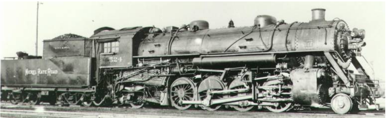
NKP 524 in 1951. New tender, new cab, new pilot, Mar's light, second turbo generator slant mounted on the engineer's side, and a muffler. The engine should also sport a low water alarm on the fireman's side.
