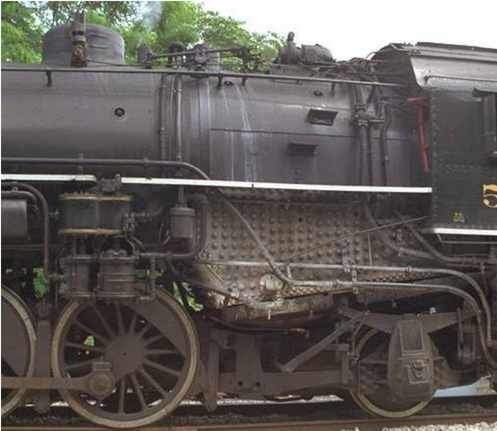
587's fireman's side boiler rear piping
