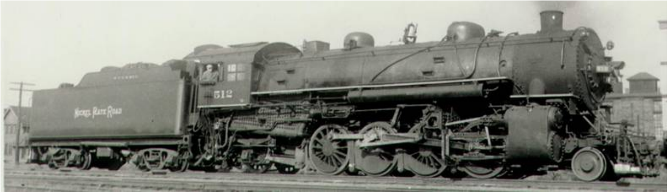
NKP 512 in 1939, pretty much as built. Only the pilot has been changed,
