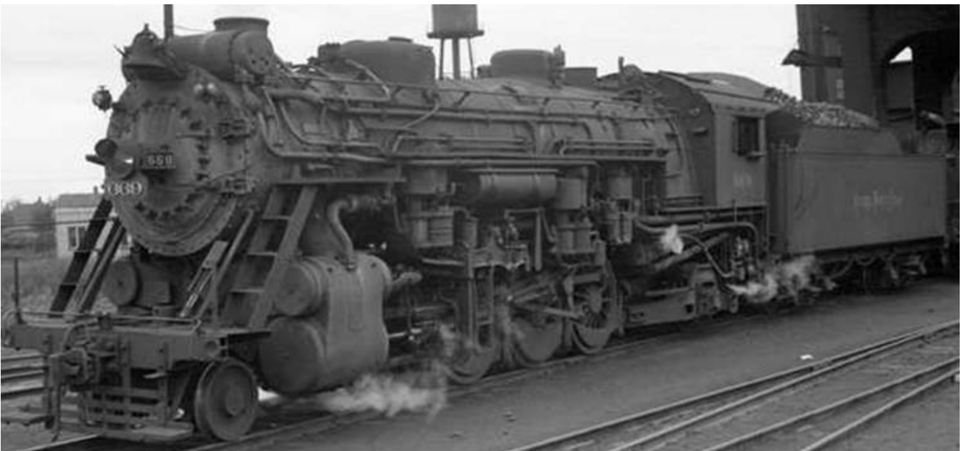
NKP 669, Conneaut, 8/24/33. Another view of an as-built H-6f. Note that both of the above engines have significantly more piping on the fireman's side than on the engineer's, and that the engines do not have a third air tank on the pilot deck. By 1929, some of the engines started receiving minor upgrading, mostly by moving the air pumps to the pilot deck (to improve the engine's balance) and the addition of blow-down mufflers and Barco low-water alarms.
