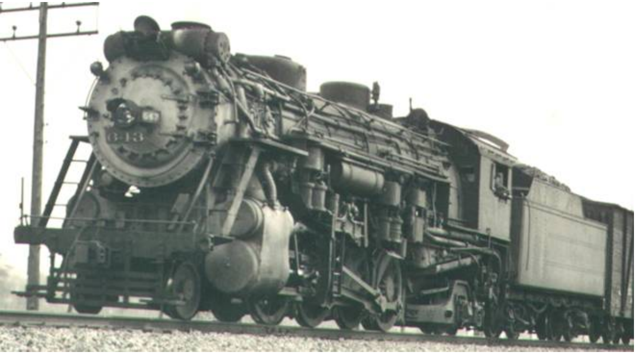
NKP 643, 1931. With the exception of the new, larger cab, this engine is pretty much stock. Note all the hardware on the fireman's side of the engine, which is what made these engines ride off-balance and rough. Also note that the smokebox is painted light graphite, a relatively short-lived system wide application that only survived past 1945 on the Pacifics and Hudsons.
