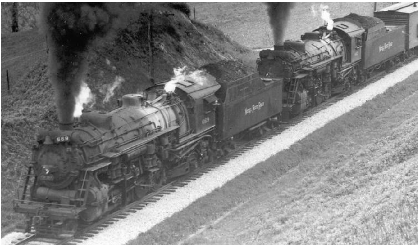
A great shot (cropped up; sorry!) of H-6f’s 669 and 667, in Indiana just after WWII. Neither engine has had their air pumps moved (and never will), but they still have minor variations nonetheless. 669 has flying number boards, a standard four slat pilot, and its original tender (with coal bunker extensions). 667 doesn’t have the new numberboards, has a sheet steel pilot, and has a larger 13RA tender. Both engines have different steam turret piping arrangements as well. Oh, and the grabs above the cab windows each have different numbers of braces.
