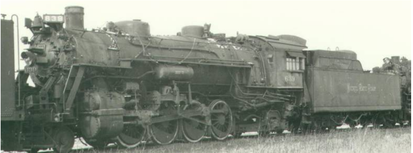
NKP 639, in the dead line at Bellevue, 1958. This is what an H-6e looked like shortly before retirement. This engine has lost its booster, feedwater heater, third air tank, and most of their resultant piping. By the end of their careers, these engines looked pretty naked.
