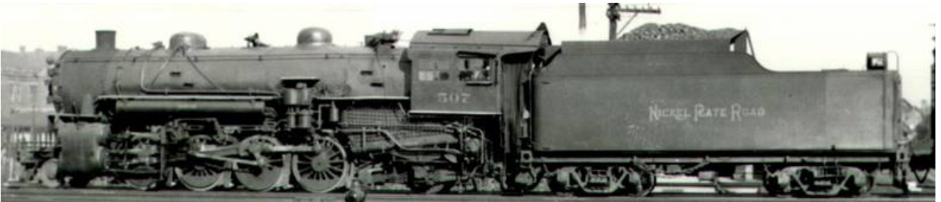
NKP 507 circa 1940. The engine still has its original cab & pilot, but the tender coal bunker has been enlarged.
