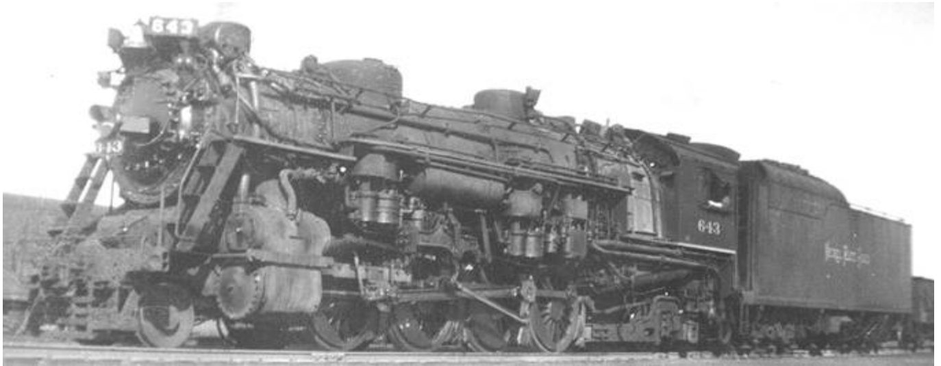
NKP 643. This engine has received multiple-bearing crossheads and flying numberboards. 643 was one of the few engines of this class to never have the air pumps moved to the tender deck (there's a large auxiliary air tank in place on the deck instead).
