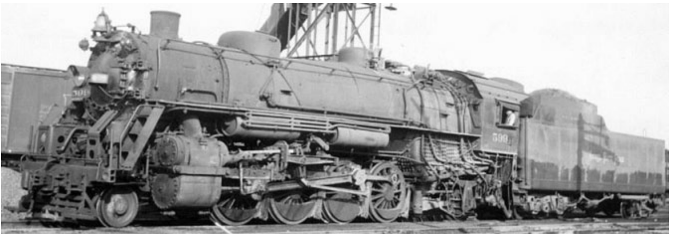
NKP 599, Delphos, date unknown. This is how the four engines which had their air pumps moved to the pilot deck looked before the addition of the Worthington feedwater heaters. Note that a four-slat pilot has been added, as well as multiple-bearing crossheads.
