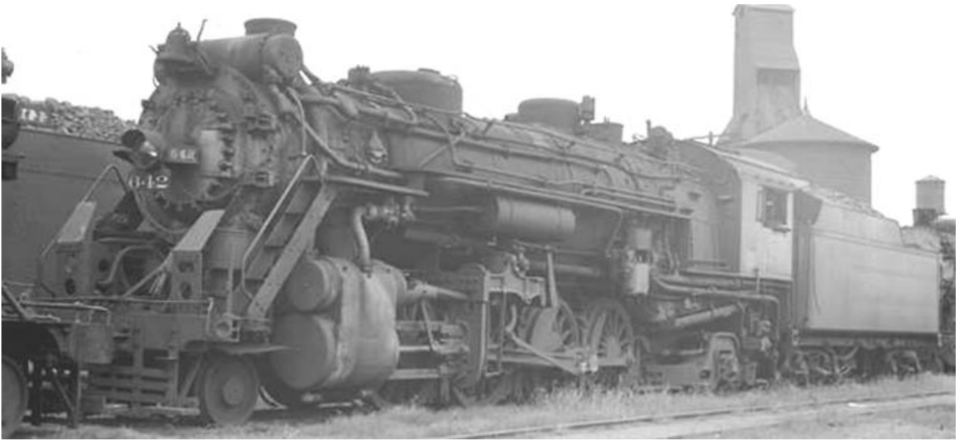
NKP 642, in storage late in the Depression. This is what the engines looked like after the air pumps were moved to the pilot deck. Some engines received a second air tank on the fireman's side, just in front of the Elesco pump.
