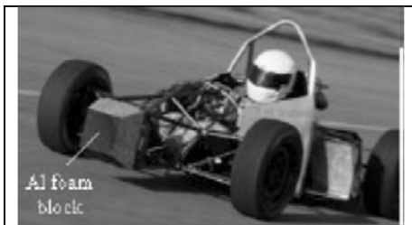
Figure 1. Race Car with "Crash Absorber" made of aluminum foam [3]
