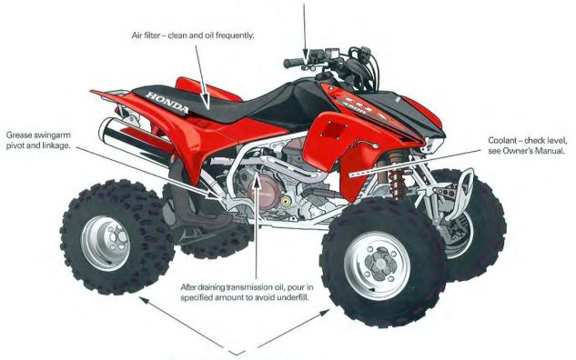
Tires – check the air pressure before every ride. Pressure gauge supplied in tool kit.
