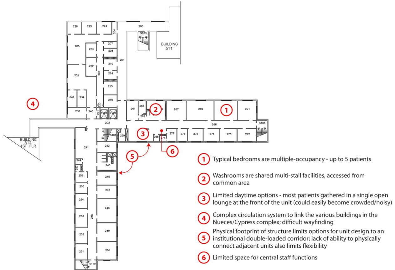
Rusk State Hospital – partial plan of the Nueces / Cypress complex, illustrating some of the challenges presented by the footprint of the building
