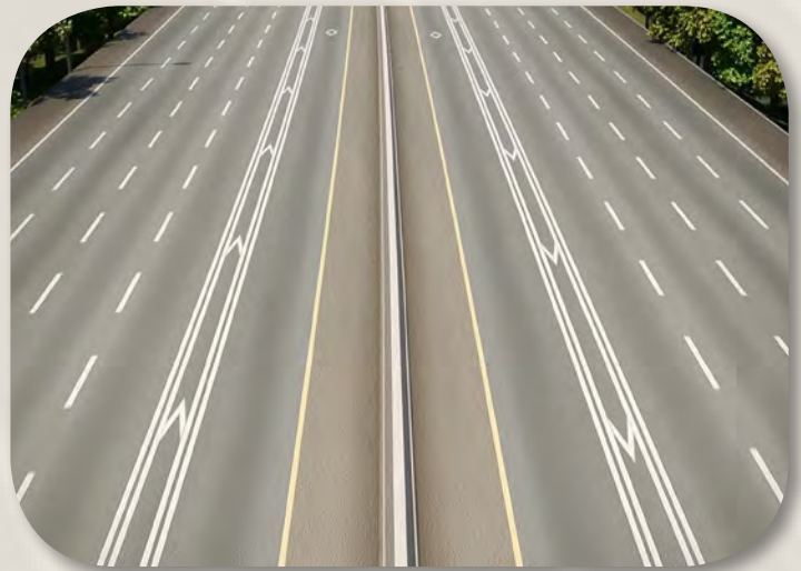
I-65 with HOV lanes on the inside and auxiliary lanes on the outside (Proposed)
