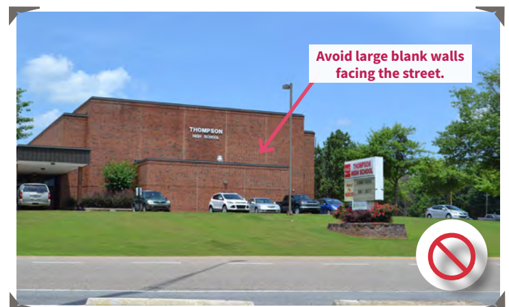
Glazing enables pedestrians to see activity on the street, and pedestrians to see what's going on inside of a building, store, or institution. This permeability is essential to creating a pedestrian oriented environment and a unique sense of place.
