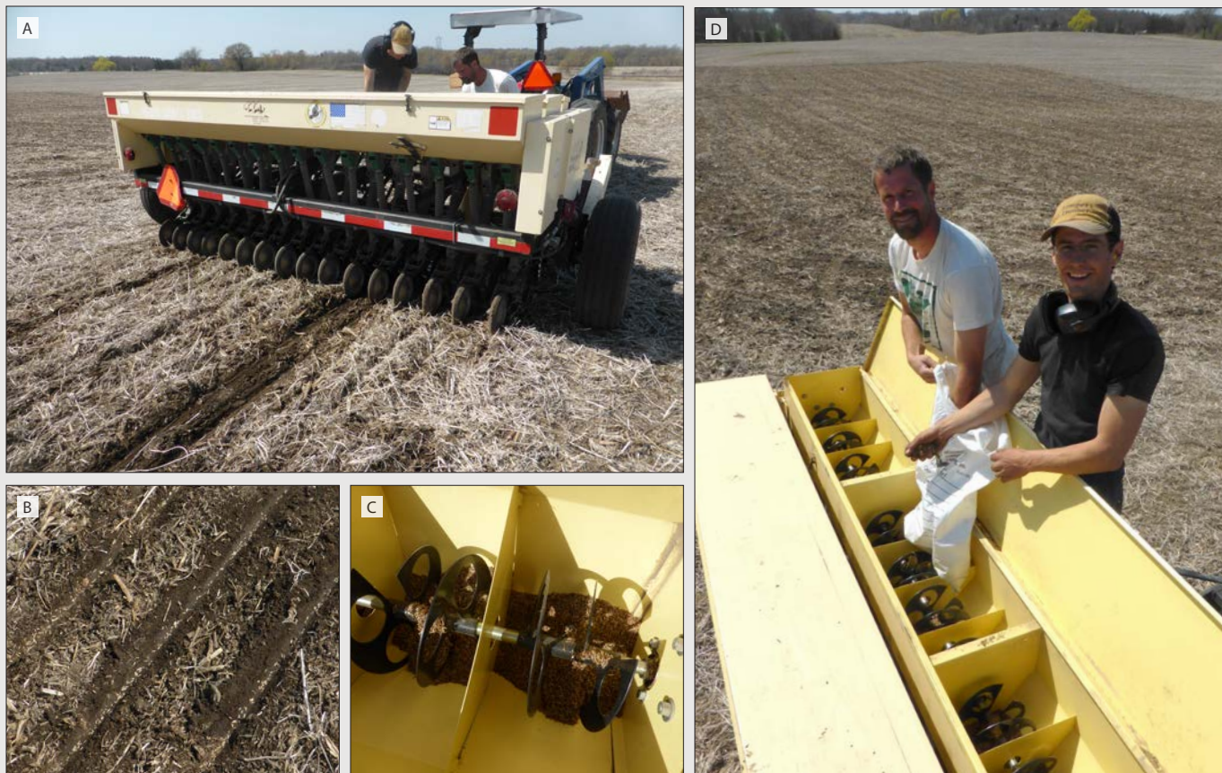
Figure 8: Native seed drills (A) are the ideal tool for large planting sites (5+ acres). Typical models can plant in a light stubble layer (B), have depth controls for optimal seed placement, and have separate seed boxes for different sizes of seed (C, D). Such drills need an experienced operator and careful calibration.
