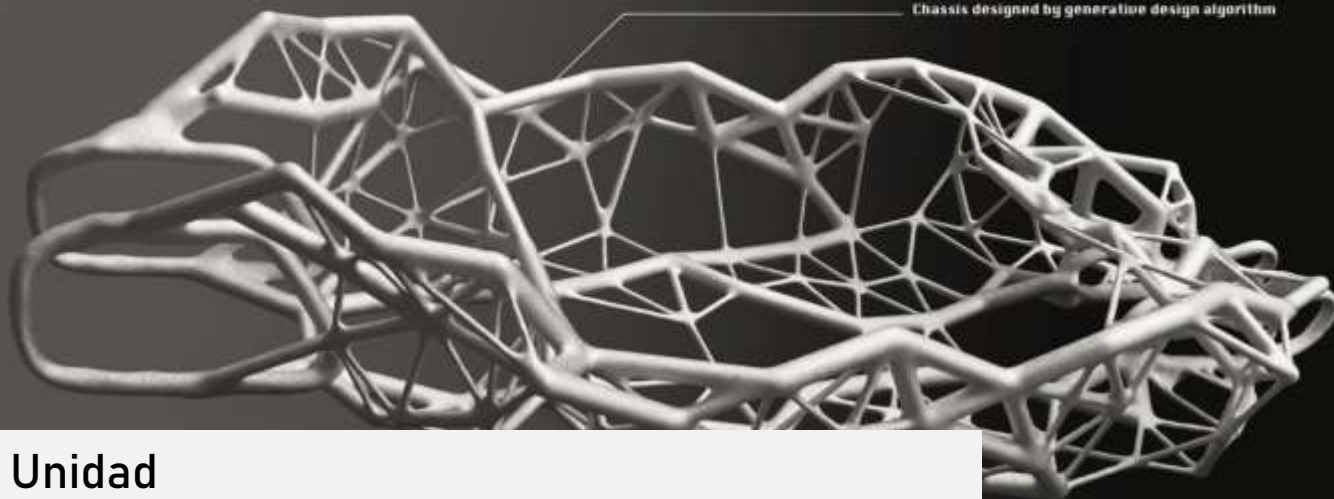
Chassis designed by generative design algorithm
