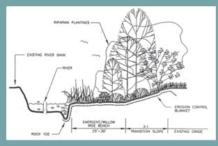
A cross-section diagram of an emergent bench approach to bank stabilization. This approach creates a gentler bank slope, allowing for both steam toe protection as well a habitat using rock and nativ riparian vegetation to preven erosion.
