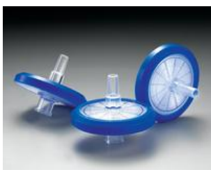
Figure 4. Disposable 0.45 \mu\text{m} filters used with syringe when filtering water samples.
