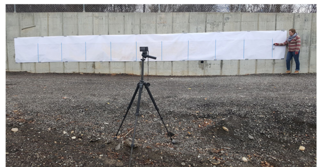
Figure 3. Setup for documenting bear spray velocities, distance, and time. High-speed camera in foreground recorded 960 frames/second, allowing the calculation of velocity from recorded distance and time for spray.
