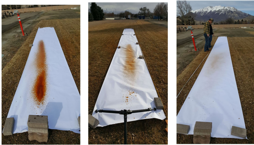
Figure 7. Spray plume dispersion as a function of temperature. The left image is of bear spray chilled to -23^{\circ}\text{C} , the center image is of bear spray chilled to -17^{\circ}\text{C} , and the right image is of bear spray at 18^{\circ}\text{C} .
