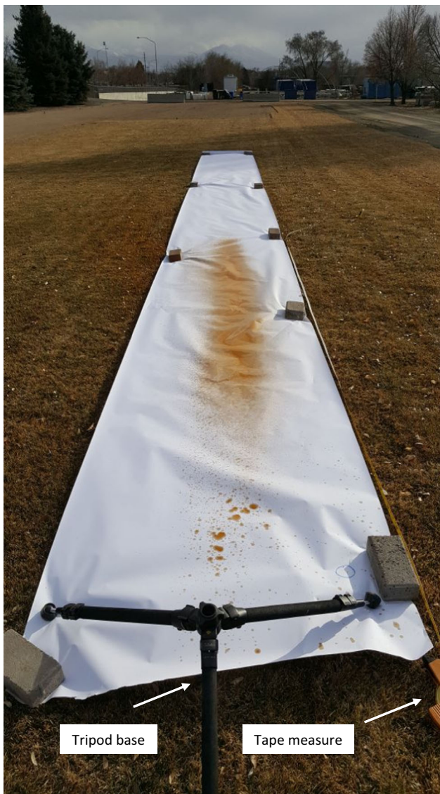
Figure 2. Field testing of bear spray distance and dispersion as a function of canister temperature. Bear spray was placed atop the tripod in the foreground, putting the nozzle at 50 cm above the ground.
