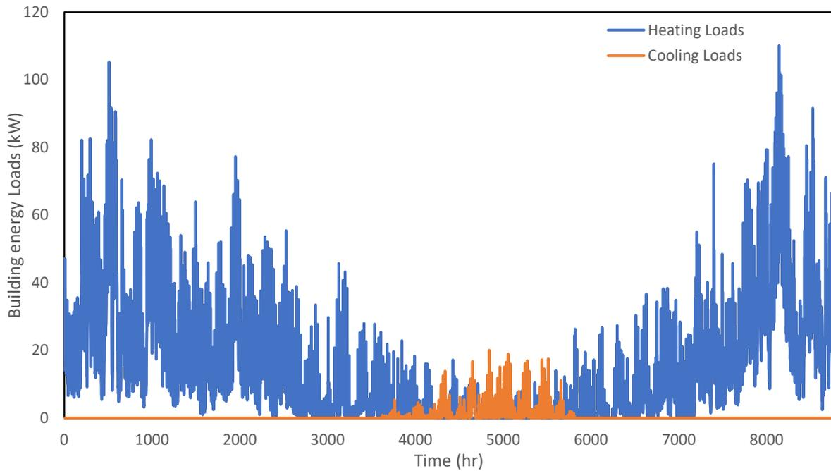
**Figure 9.** Hourly heating and cooling energy loads for the apartment building
