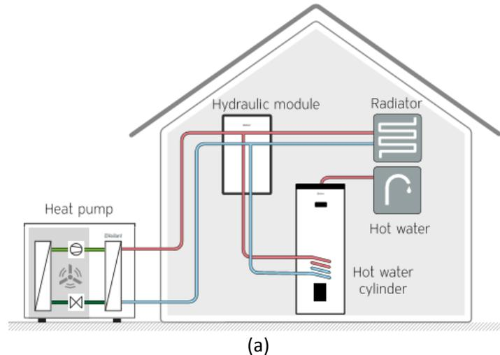
**Figure 13.** (a) Schematics of an ASHP system (BioSun Energy, 2023)
