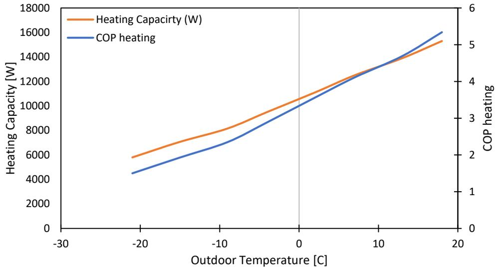
**Figure 14.** COP heating and heating capacity of the chosen ASHP vs. outdoor temperature
