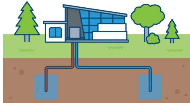
**Figure 16.** Schematics of an open loop ground source heat pump system or ground water heat pump system (Efficiency Manitoba, 2021)
