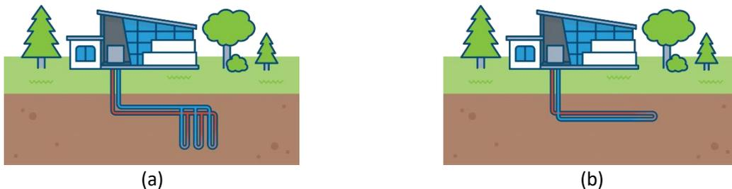
**Figure 18.** Schematics of a closed loop ground source heat pump system: (a) vertical (b) horizontal (Efficiency Manitoba, 2021)
