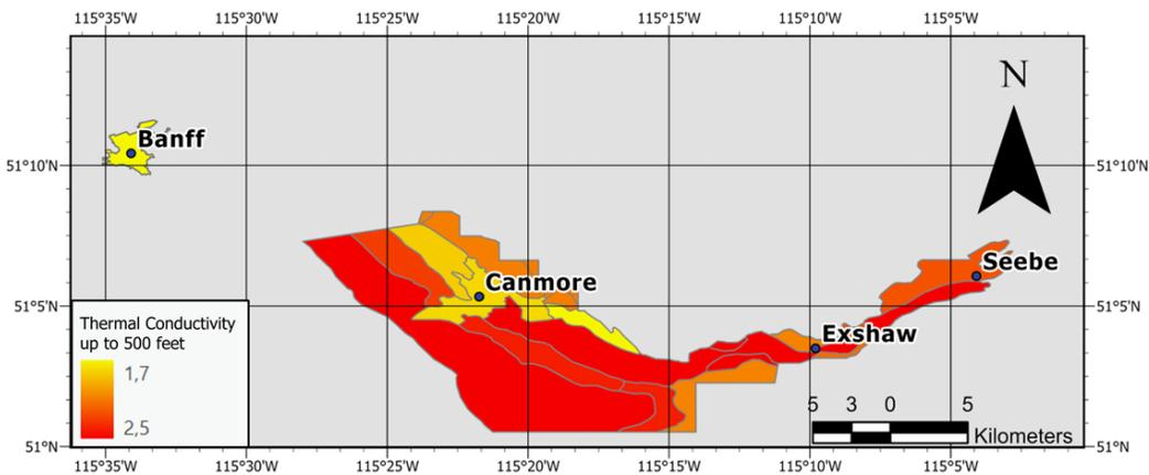
**Figure 4.** Thermal conductivity results for up to 500 feet. Values given in W/mk.
