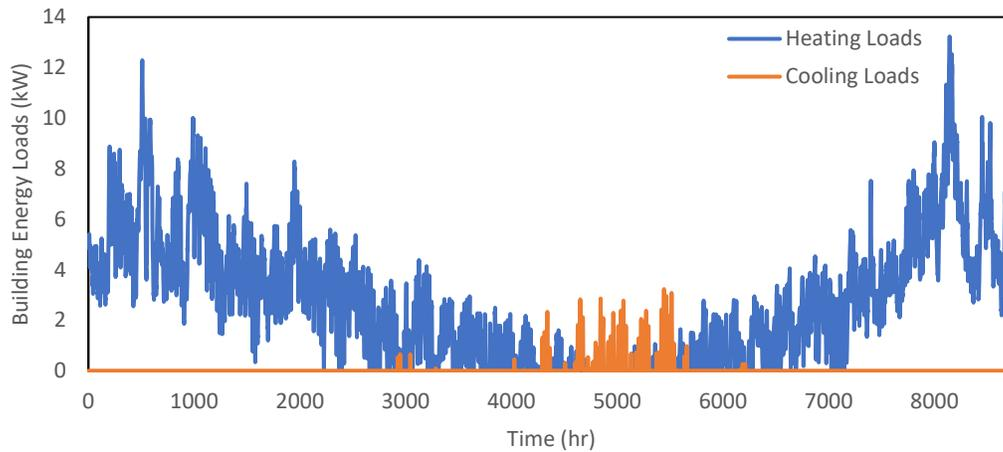
**Figure 7.** Hourly heating and cooling energy loads for the detached multi-family building
