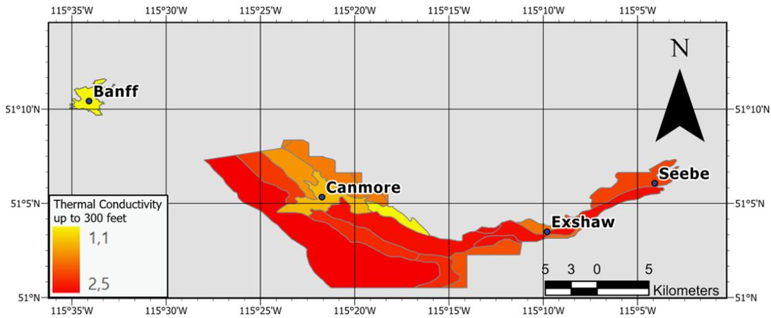
**Figure 3.** Thermal conductivity results for up to 300 feet. Values given in W/mk.
