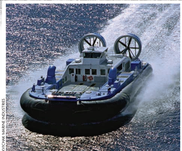
The 98-foot Suna-X Hovercraft Ferry has completed more than 30 successful medevacs between King Cove and Cold Bay. Based on historical weather data for the bay, the craft should be operational 99% of the time, whereas the proposed 30-mile gravel road through refuge wilderness would be dangerous and totally unreliable in drifting snow (see cover photo).
