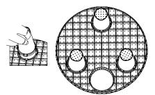
**b.** Insert the brine well assembly inside the grid plate as well below.
