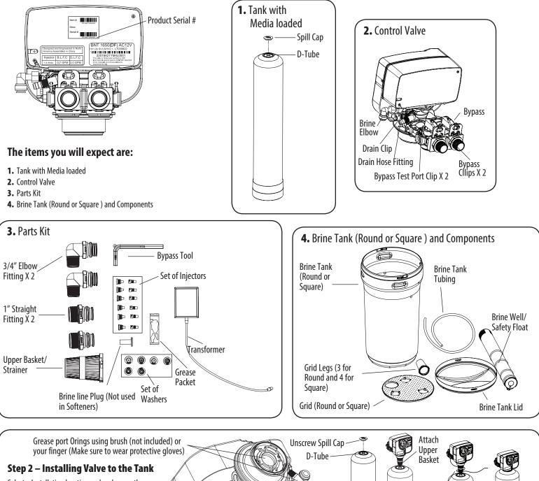
Select a Installation location and make sure there is access to 110V power outlet and drain line. Lube the bottom Valve Orings with the grease supplied, Attach the Upper Basket. Unscrew the spill cap. Carefully Slide the D-Tube inside the Valve and Screw the Valve inside the Tank such that the power cord doesnt get caught between the valve and the tank
