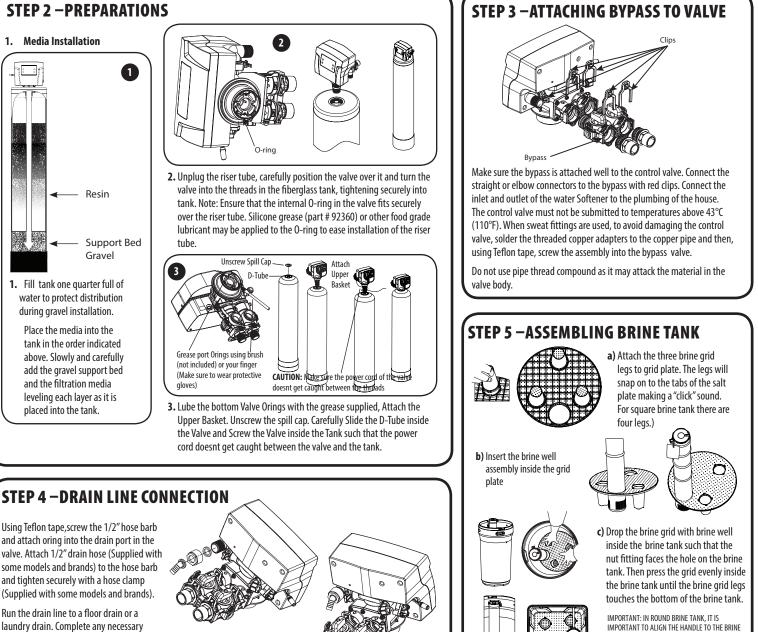
Run the drain line to a floor drain or a laundry drain. Complete any necessary plumbing.
