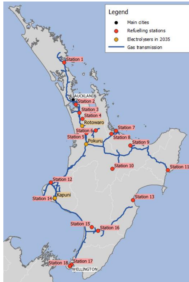
Electrolyser locations in 2035: Additional sites for injection of hydrogen into the transmission network (20% by volume) hydrogen blend
