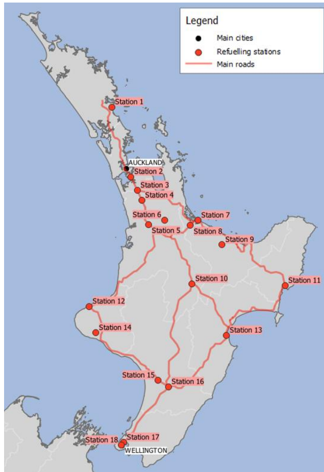
Refuelling station hub locations: Sites for onsite electrolyzers to meet transport demands
