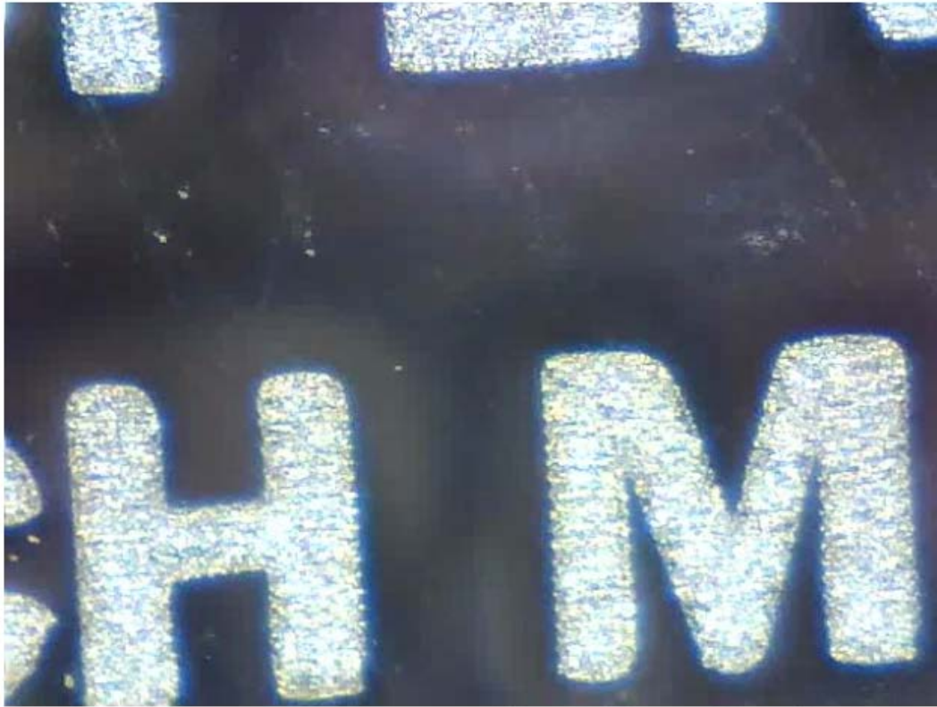
Caption: Low-quality microscope image showing 1 micron tall letters etched into a nickel layer of the analog layers, of the Lunar Library™ -- with more powerful microscope the letters can be seen to have very defined and clear edges
