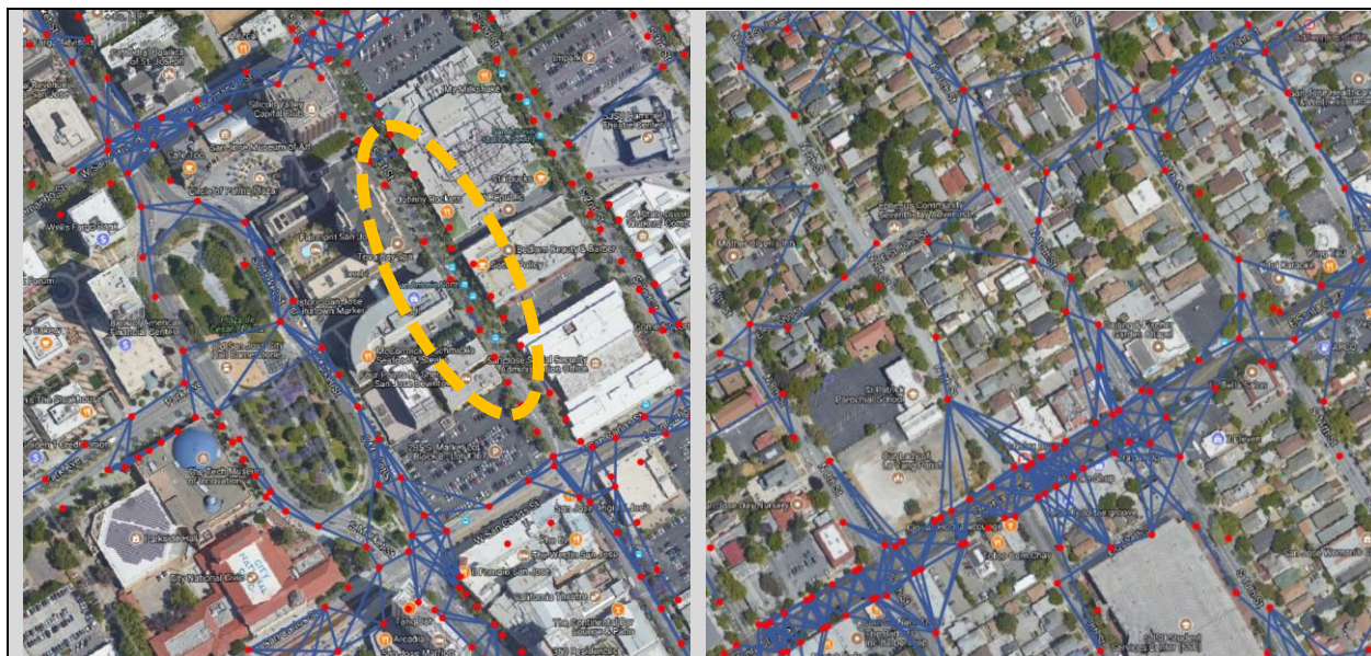
FIGURE 3 LOS COMBINATIONS, RED DOTS: STREET LIGHTS, BLUE LINES: LOS LINKS, YELLOW: LOS BLOCKED BY TREES
