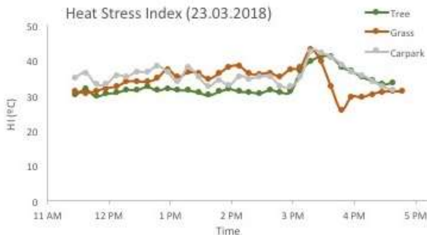
Figure 22. The Heat Stress Index (HI) for the treed (shaded), open grassed, and carpark (sealed) sites on 23 March 2018.
