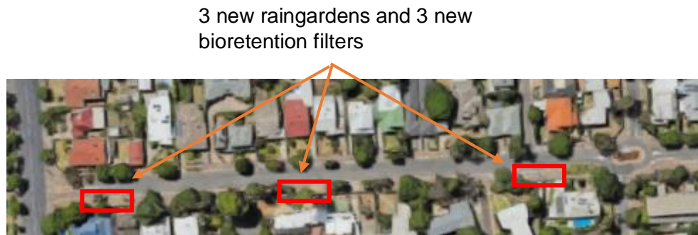
Figure 5: The study area and its surrounds, prior to implementation of WSUD and GI features.
