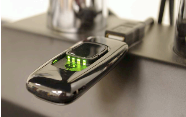
Fig. 2. The clip on activity monitors used in the study plugged into the USB port of the Kiosk. The USB interface on the activity monitor is retractable.
