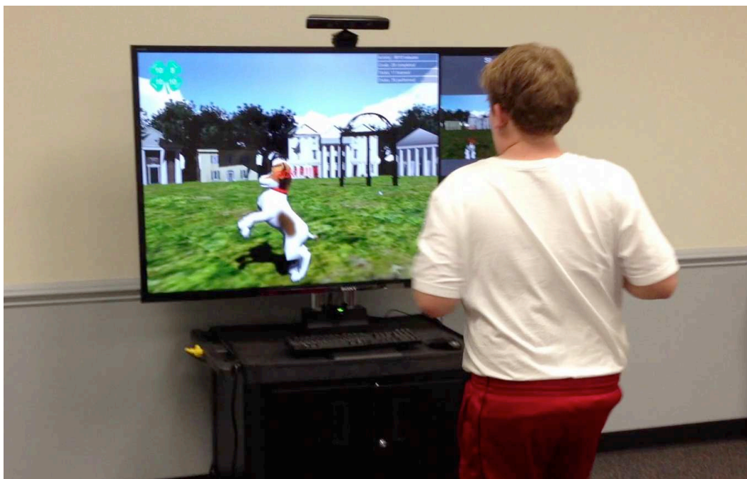
Fig. 1. A child interacts using speech and gestures with a mixed reality virtual pet kiosk. A wearable USB activity monitor is currently plugged into the kiosk that identifies the user and allows real world physical activity to serve as input into the simulation.
