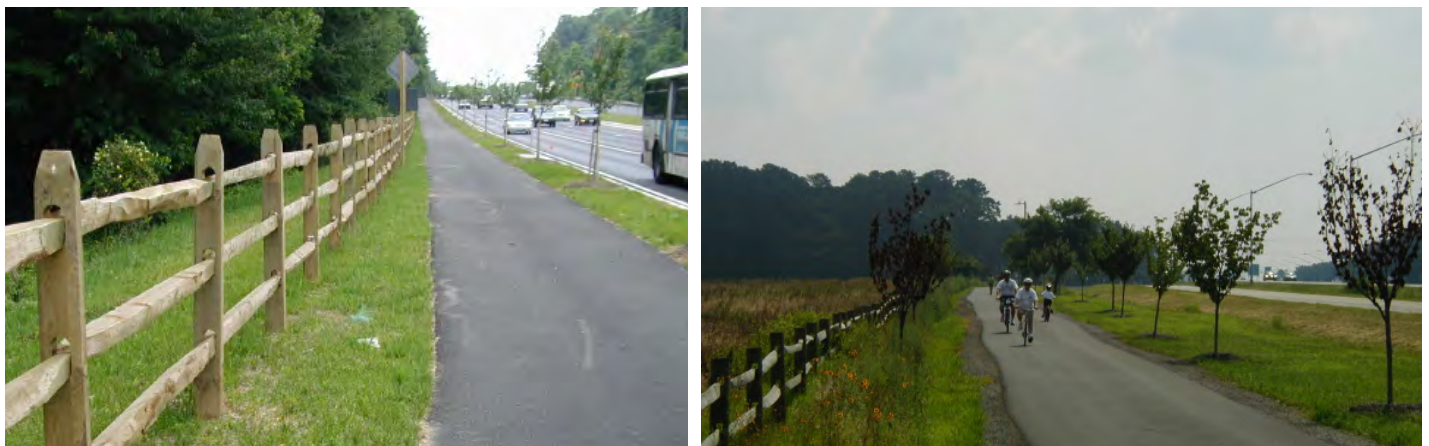
Adequate buffer space between the trail and the roadway provides a comfortable and appealing facility for a variety of trail users.
