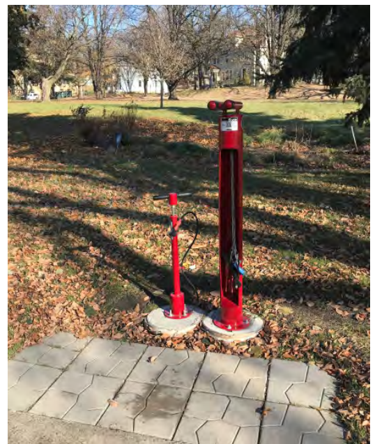
Bicycle repair stations provide quick access to bicycle repair tools for trail users, such as wrenches, screw drivers, and air pumps.
