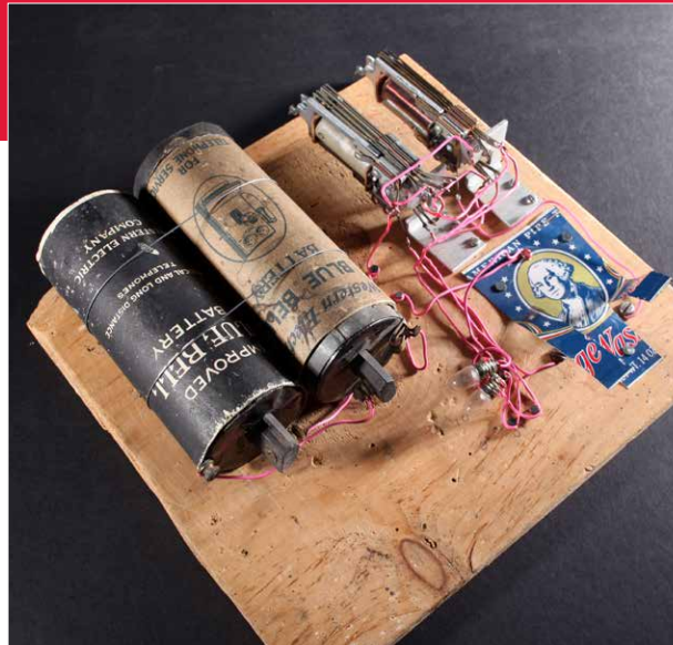
Model K binary adder built by Dr. George Stibitz, ACRM Collection Shawn Raecke photo
