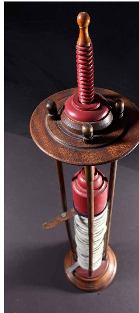
Volta Pile manufactured in Italy circa 1800, ACRM Collection Shawn Raecke photo
