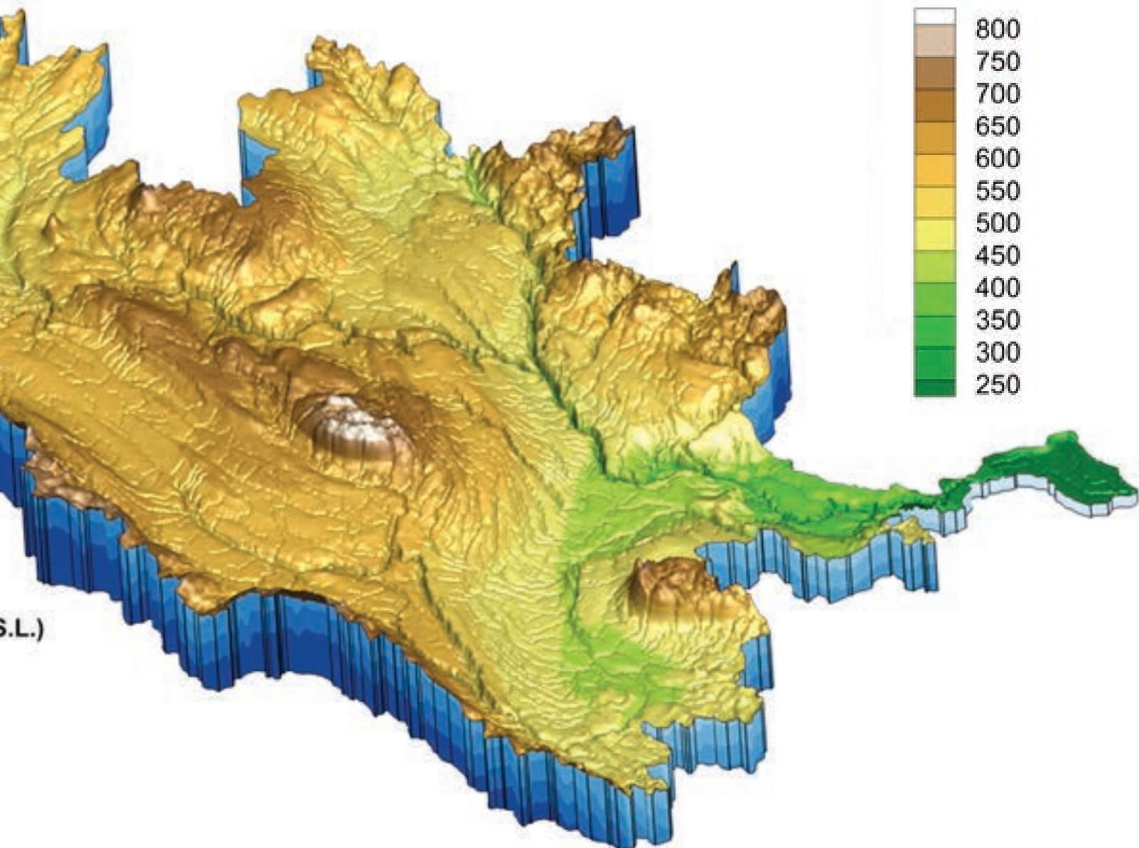
Key physical and hydrologic features of the Assiniboine River Basin are represented digitally in the 3D framework (inset A) of the HydroGeoSphere model, including the major surface water operational structures (inset B), and topography and ground-water (main image)
