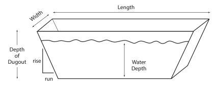
The dugout calculator uses the following formula for a prismoid to calculate the volume.
