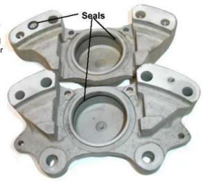
The next step I did was to powder coat the caliper halves. One could follow the same process if painting the caliper. The rubber seals were removed from the inside of the cylinders, as was the little rubber washer seal between the two caliper halves. All the holes were plugged and old pistons were inserted into the cylinders to keep the paint out of there and the machined surfaces where the two haves mate were carefully masked. The photos below show the powder coated halves of one caliper.
