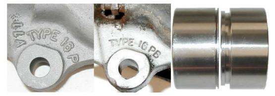
**Piston Boots:** The early pistons have the narrow groove as shown above. The edge of the boot fits into the groove. The other side of the boot rides on the side of the piston. The boot is shaped such that it naturally spreads toward the front edge of the cylinder to complete a sort of seal. The photo on right shows such a boot installed on an early piston.
