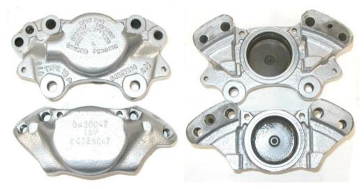
The next thing I did was run a tap though all threaded passages and then blow out all passages. I then covered the cylinder with a light coat of brake fluid. It is very important that no petroleum based grease or oil get into the brake system so only brake fluid and the Girling or Lockheed Rubber grease were used on the parts.
