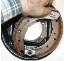
I next hook one end of the top spring into the top hole in the front shoe and then grasp the top of the rear shoe with pliers as shown on the right. The rear shoe is lifted off the wheel cylinder and brought to the front far enough to hook the back of the top spring into the top hole in the rear shoe. The pliers are then used to gain extra leverage to push the top of the rear shoe to the rear far enough so that it can be positioned in the back of the wheel cylinder.
