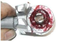
The next step was to install the dust cover and dust cover retainer as shown on right. The final step was to coat the threads on the bleed nipple with the red rubber grease, install the nipple and then the bleed nipple cap. It'll be at least a year before these see service so it's import to close the input port. I temporarily used silicone plug from my powder coating masking kit. After everything is installed I plan to plug the hole with a short 3/8-24 bolt.
