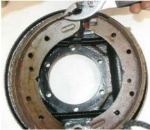
The last step is to push the shoe retaining pins in from the rear and secure with the shoe hold down springs. I chose not to
