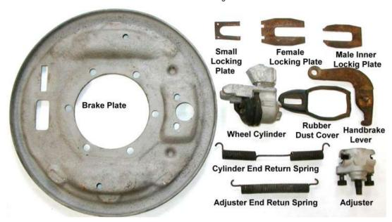
**Disassembling Adjuster & Wheel Cylinder:** The adjuster came apart pretty easy this time. In the past however I've had trouble freeing the adjuster screw. A shot of PB Blaster, and overnight wait and then heating with a propane torch seems to free the steel parts from the grasp of the aluminum castings. I usually don't want to wait so give it a shot of PB Blaster --- get a cup of coffee --- heat --- PB Blaster, heat again, at which point it usually comes free.
