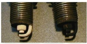
The brownish color over the tip and part of the center porcelain on the left plug indicates a carb with proper mixture. The uniform more whitish color of the right plug indicates a carb that the mixture is still a little lean.
